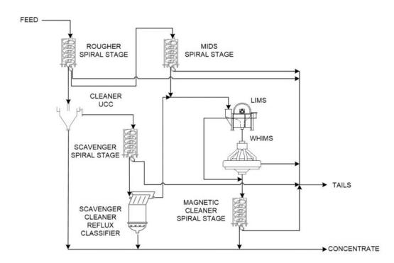
In each concentrator, the classification screen pumps feed four primary distributors that evenly distribute the feed to each of the 32 rougher spirals feed distributors. The rougher spirals feed distributors then redistribute the feed to each of the spiral starts of each rougher spirals bank. There are 40 spiral starts per bank in Phase I and 36 starts per bank in Phase II.
